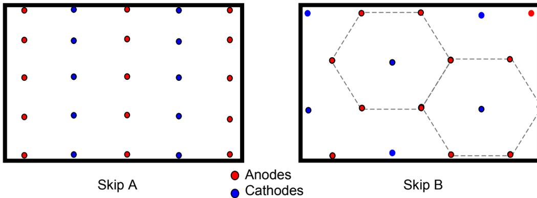
FIGURE 1 – ELECTRODE ARRAYS IN SKIPS A AND B
