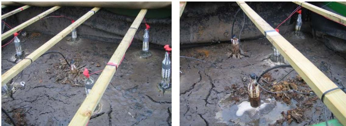
**FIGURE 2 SKIP B HEXAGONAL ARRAY SHOWING EFFECTIVE SIPHON DEWATERING ON THE LEFT AND INEFFECTIVE SIPHON DEWATERING ON THE RIGHT.**
