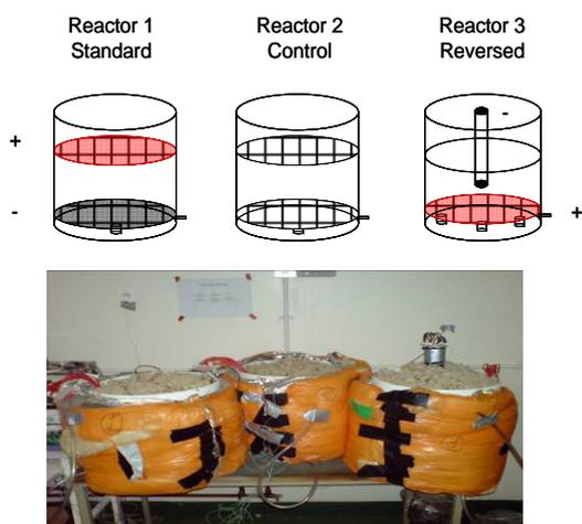
**Figure 1.** The laboratory trial set up showing the three separate reactors. From left to right reactor 1 is the ‘normal’ polarity set up, reactor 2 is the control & reactor 3 is the reverse polarity set up.
