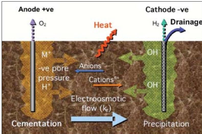
Fig 2. Summary of the relevant processes during electrokinetic ground treatment.
