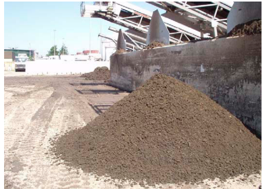
Figure 2 Sewage sludge at 30% dry solids and 50% volume reduction
