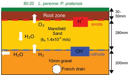
Figure 6. Profile of suspended water table pitch.
