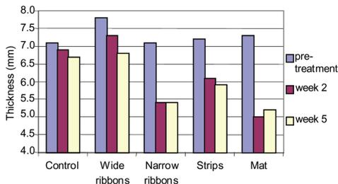
Figure 5. Thatch thickness measured before during and after electrokinetic treatment.
