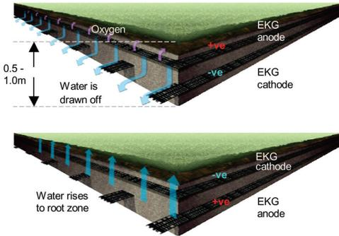
Figure 2. Conceptual model of EKG-turf system. Upper: normal polarity. Lower: reverse polarity.
